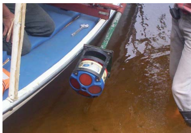
Figure I.5.4. Transducer of an acoustic Doppler instrument installed on a boat
