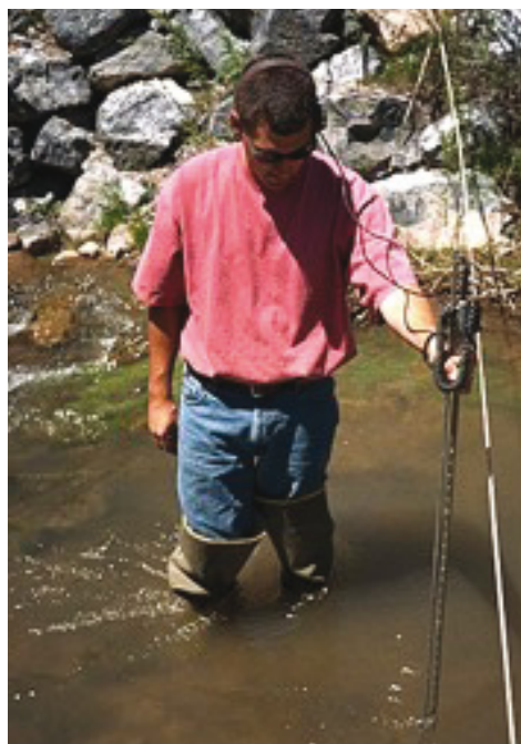
Figure I.5.67. Wading measurement using a top-setting rod
