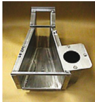
Figure I.8.3. Plans for modified 3-inch Parshall flume
