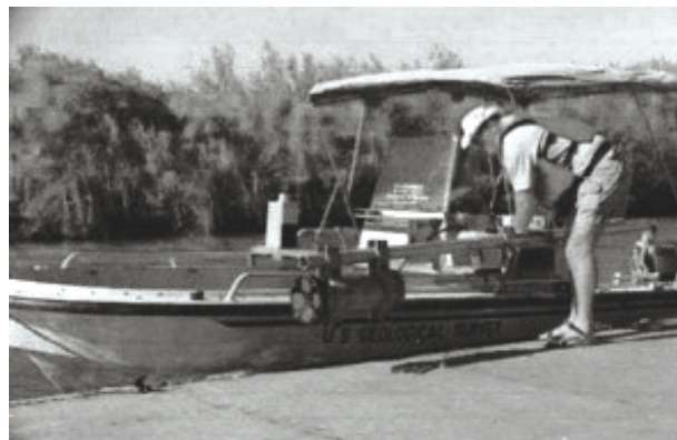
Figure I.6.11. Side-swing mount on a 6-metre Boston Whaler for an ADCP
