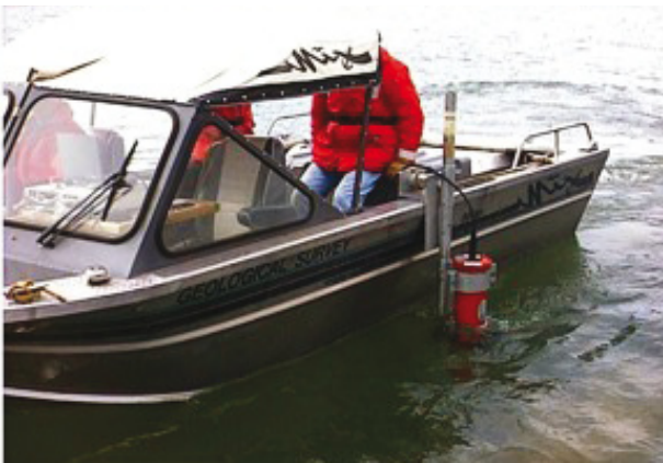
Figure I.6.17. Side-mounted ADCP mounting brackets
