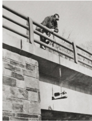
Figure I.5.52. Measuring from a bridge with a handline
