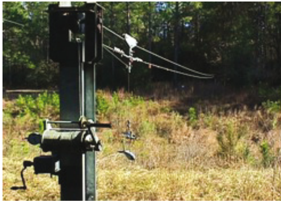
Figure I.5.51. Remotely operated cable car assembly
