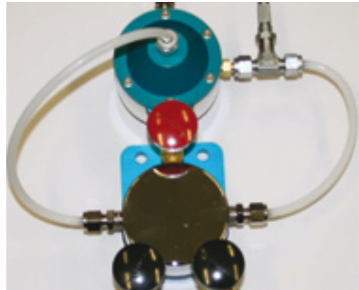
Figure I.4.25. Hydrological Services Model HS-23 dry bubble gas purge unit
