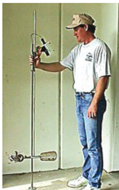
Figure I.5.24. Top-setting wading rod with meter attached
