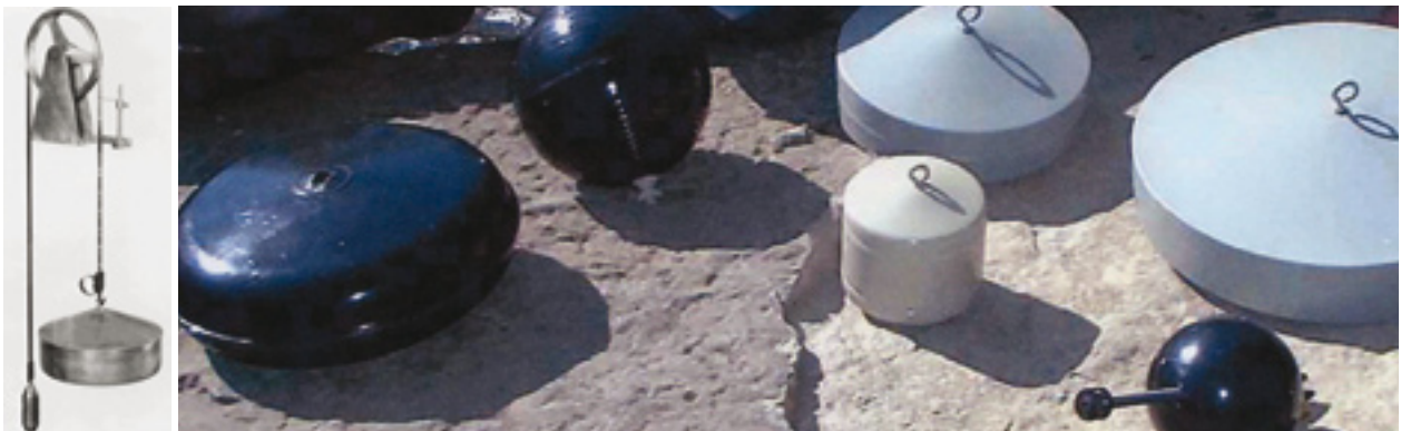
Figure I.4.19. Float-tape gauge and various float types
