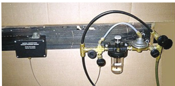
Figure I.4.27. Sutron Accububbler model 5600-0131-1 self-contained gas-purge system
