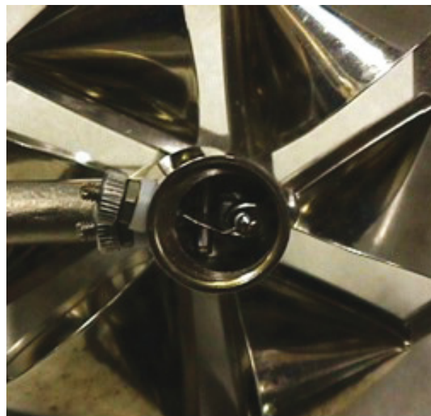
Figure I.5.12. Contact chambers for cat whisker heads and magnetic heads
