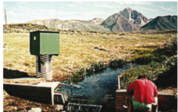
Figure I.3.2. A suppressed rectangular weir
