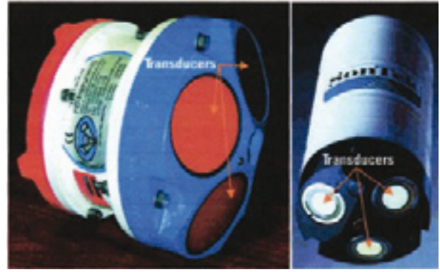
Figure I.6.8. Two Acoustic Doppler Current Profilers, an RD Instruments Rio Grande (left) and a SonTek model (right)
