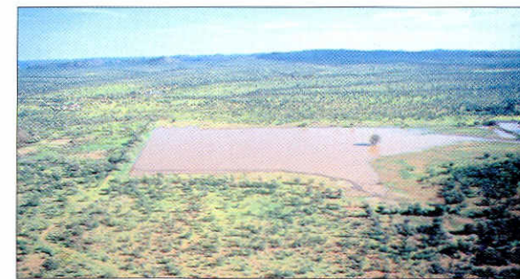
Farm dams, such as this one in the upper Huab catchment, occur throughout the western catchments. Although they provide water for stock farmers in the headwaters, they also reduce downstream flow. When added together over an entire catchment, such dams may have a major effect on the downstream environment. Large numbers of ana trees are dying in the upper Huab catchment, due to the combined effects of farm dams and decreased rainfall. Although needed, no thorough study has been conducted to accurately determine the effect that such dams have on runoff patterns throughout the western catchments.
