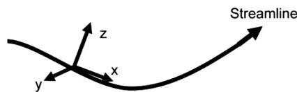
Figure 5.2 Schematic presentation of the coordinate system ( x, y, z ), with the x-axis parallel to the flow direction.
