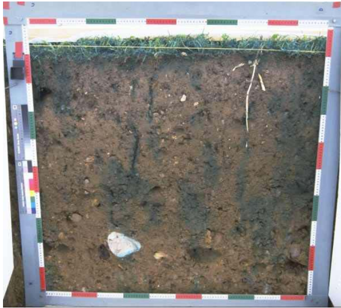
Figure 5. (a) Photograph of cross section through soil following dye tracing experiment (Courtesy of Markus Weiler).
